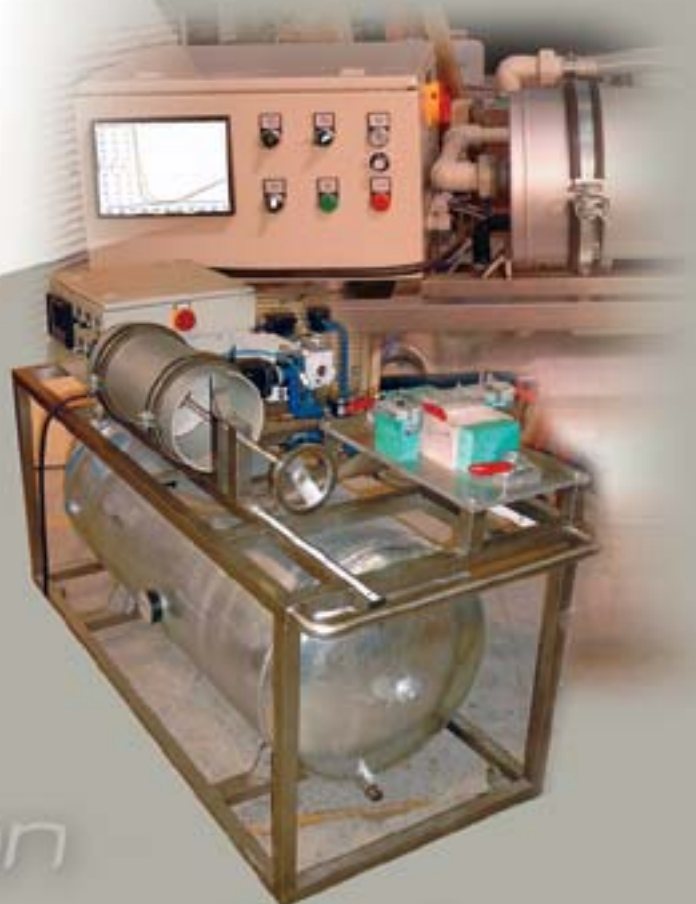
Vacuum test stand Volume up to 20.000 ccm
